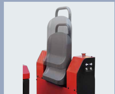
Backrest height can be adjusted within a certain range, and the backrest with hip support can greatly improve the comfort of the operator
